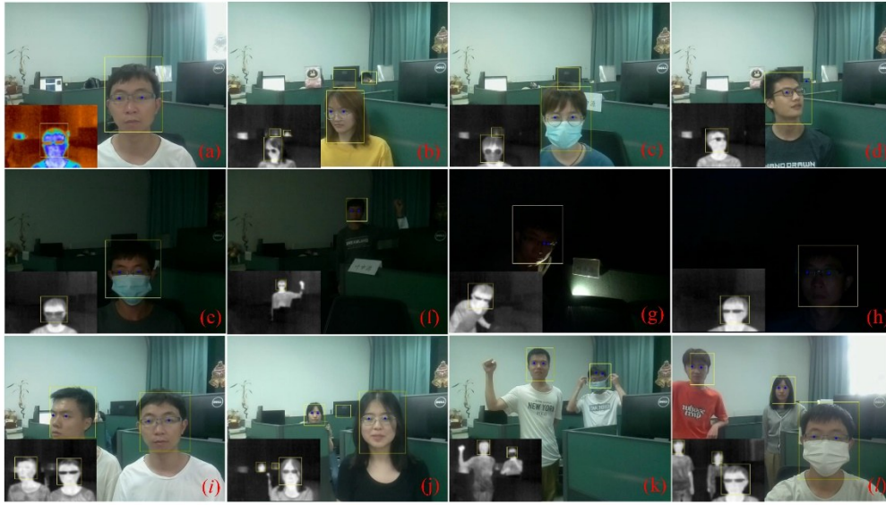
Fig. 5 IR face detection samples of YOLO-Fastest-IR and eye localization in the RGB images results; (a~d) YOLO-Fastest-IR and YOLO-Fastest-Eye is robust against angle of face inter-viewer occlusion, environmental occlusion; (e~h) extreme lighting condition; (i~l) multi target and distant viewers.
