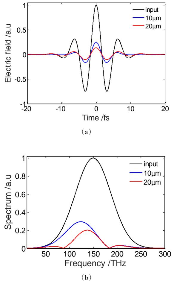
Fig. 3 The pulse distortions of few-cycle laser pulse with a wavelength of 2  $\mu\text{m}$  induced by the EOS with different thicknesses: (a) shows the time waveforms and (b) shows their frequency spectra, respectively
