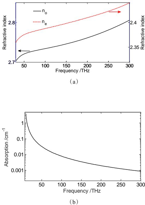
Fig. 1 (a) The ordinary and extraordinary light refractive indexes and (b) the absorption of GaSe crystal in the mid-infrared range
