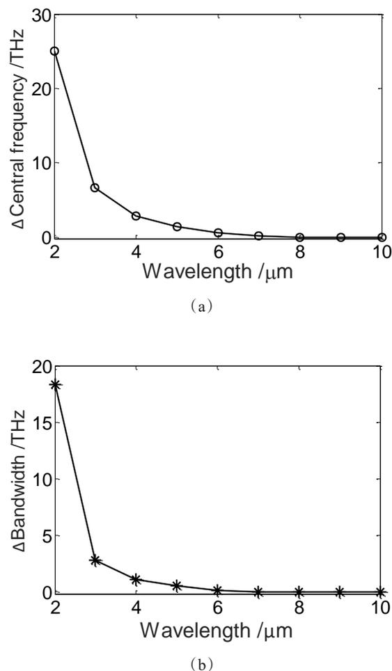
Fig. 5 The changing of (a) the central frequency and (b) the bandwidth depending on the wavelength of the few-cycle laser pulse from 2 μm to 10 μm
