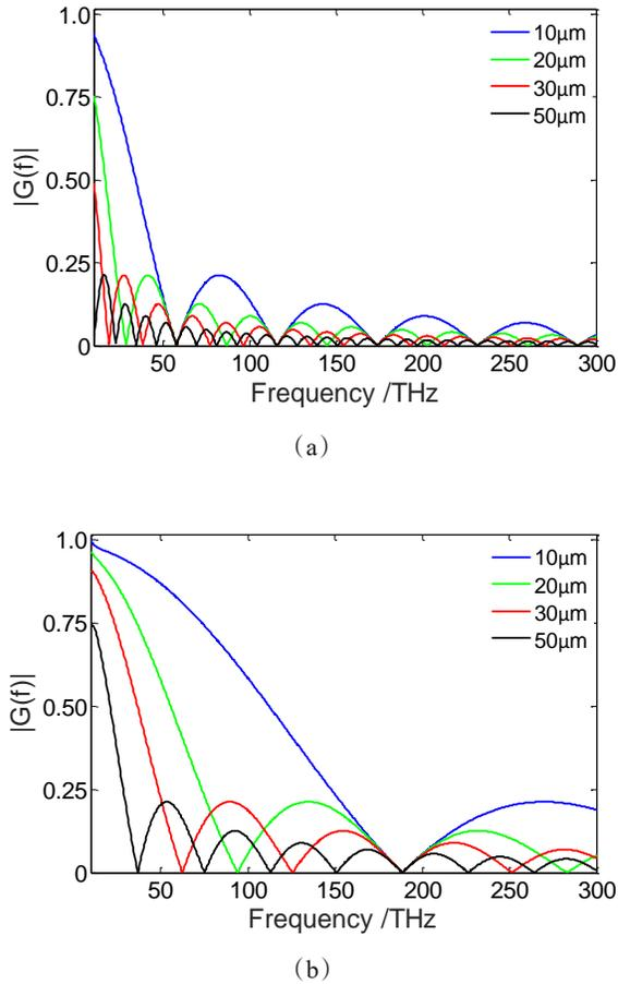
Fig. 2 The response function of the EOS with different GaSe thicknesses (10  $\mu\text{m}$ , 20  $\mu\text{m}$ , 30  $\mu\text{m}$ , and 50  $\mu\text{m}$ ) with two different probe laser wavelengths: (a) is with 800 nm and (b) is with 1030 nm
